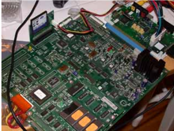
CF to IDE adapter in place on Area51 PCB (click above for larger image)
