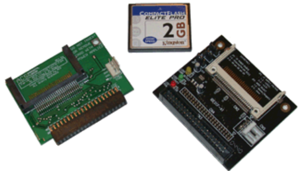
Compact Flash to IDE Adapters (direct plug-in and cabled versions)
