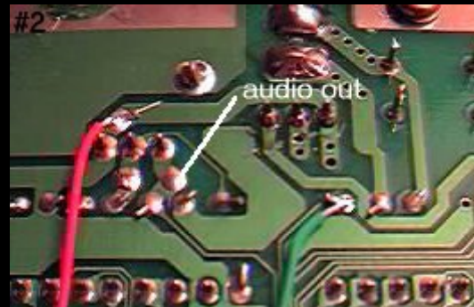
Red: +5v to amp Green: Video into RF modulator (center rear)
