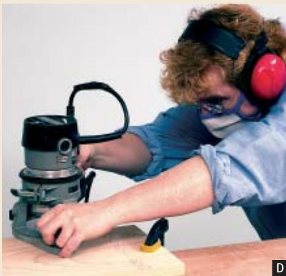
**5** Make a cut several inches long, move the bit about 1" away from the edge (as in your starting position), and turn off the router. When the bit has stopped spinning, remove the router and check the depth of cut with a sliding square. Adjust by trial and error until the depth is correct.
