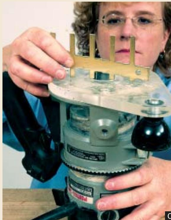
**5** Check that your workspace is clear, make sure the on/off switch is set to off, and plug in the router.
