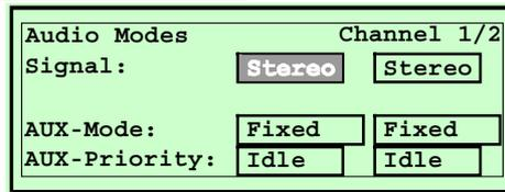
Different modes for playing of music or for the auxiliary inputs/outputs (AUX-In/AUX-Out) can be set paired for the audio channels (1/2 or 3/4).
