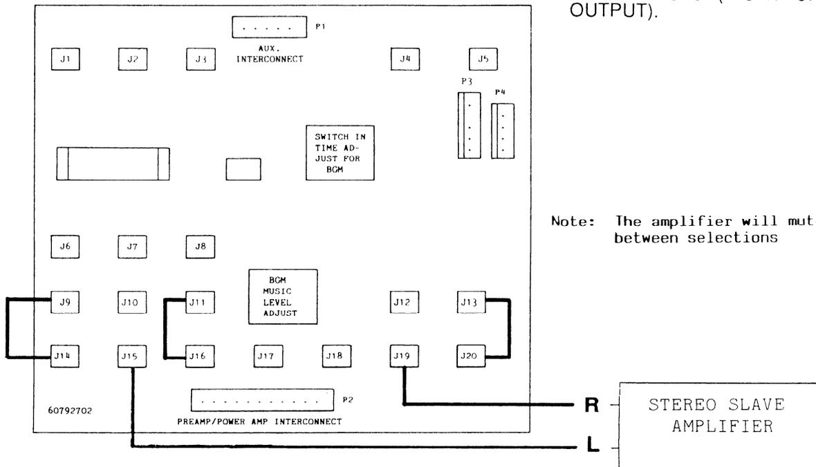
**Stereo Slave Amplifier Connections (Controlled By Phono Volume)**
