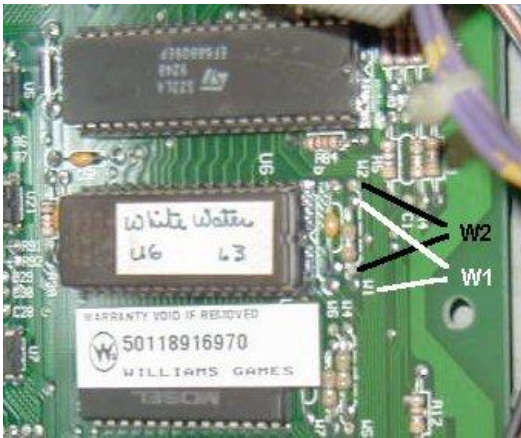
W1 and W2 removed on a WPC-89 cpu board. pic by thatpinballplace.
